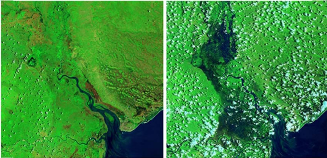
Figure 5.3 Flooding occurred in Mozambique after Hurricane Eloise in January 2021. The left image was acquired before the floods on December 27, 2019, while the right image was acquired on January 30, 2021, which shows the flooded area (dark blue). Both images were acquired by Landsat 8 OLI sensor and displayed in false color (bands 7-5-3 in RGB combination). Source: ( https://earthobservatory.nasa.gov/images/147866/eloise-floods-mozambique ).
